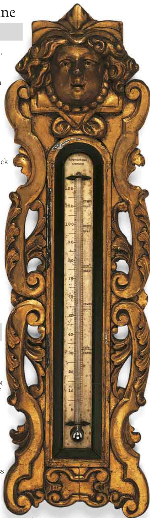
MERCURY THERMOMETER This early English thermometer has its tube attached to a scale marked on a separate piece of wood.
