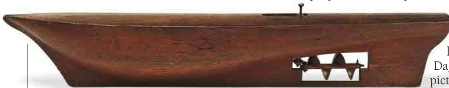
SHIP'S PROPELLER This is a model of SS Francis Smith, which was fitted with Smith's propeller. Modern ships have their propeller further back.
