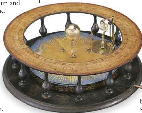
SOLAR SYSTEM Users turned the handle of this 18th-century orrery to show the annual rotation of the Earth around the Sun and the Moon's rotation around Earth.
