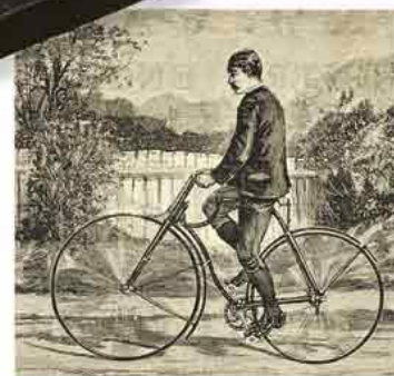
BICYCLE The Rover in this 1888 advertisement has all the essential features of a modern bike.
