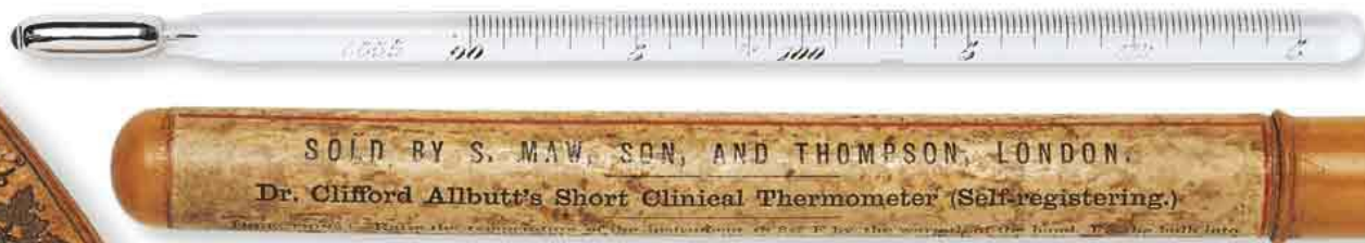
CLINICAL THERMOMETER This Allbutt-type thermometer of about 1880 looks very much like those used a century later. It was designed to hold its reading after removal from the patient.
