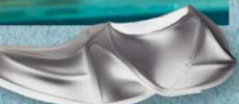
TIBBITS'S TEAM PRODUCED THE UPPER PART OF A SHOE BY PRINTING A PATTERN ONTO STRETCHED FABRIC. OVER TIME, THE FABRIC TRANSFORMED INTO THE SHAPE OF A SHOE.
