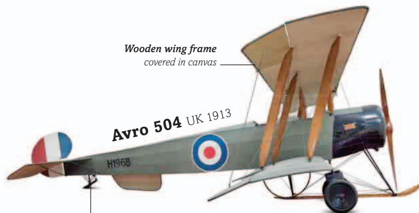
Tail skid helps slow aircraft down while landing
