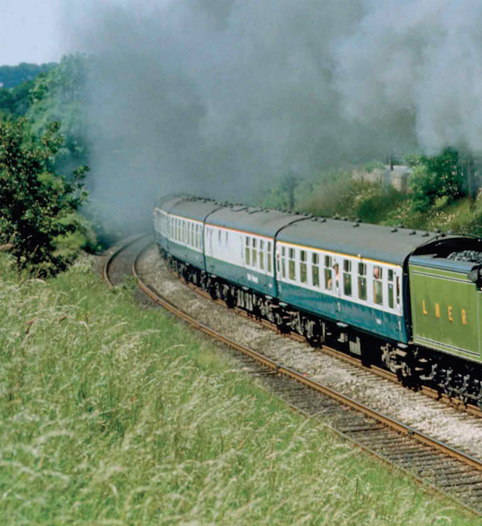
FLYING SCOTSMAN The No. 4472 Flying Scotsman powers along the tracks of the Carlisle to Settle line in the north-west of England, a service known as the “Cumbrian Mountain Express.” The 71-ft-2-in- (21.7-m-) long locomotive weighed more than 109 tons, but generated enormous pulling power. In 1934, it became the first steam locomotive officially recorded to exceed 100 mph (160 km/h).
