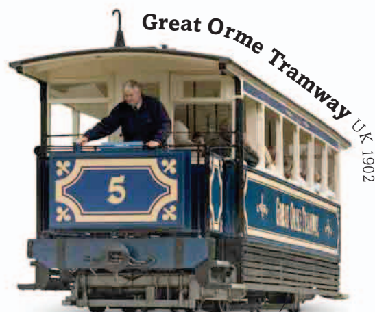
Streetcar pulled uphill by cable moved by electric motors
