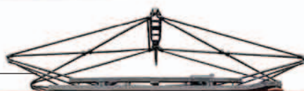
Pantograph supplies power to locomotive's three electric motors
