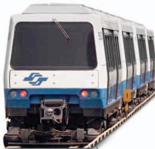
Rail supplies 750-volt electricity to power train's motors
