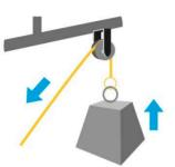
Pulley A pulley uses a rope or chain looped over a wheel to lift heavy loads.
