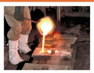
**3. Pour it in** The melted iron is poured into a shaped mould and left to cool.
