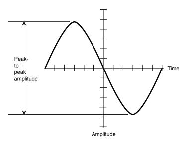
Fig. 13-11. Peak-to-peak amplitude.
