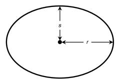
Fig. 4-34 Perimeter and area of an ellipse.
