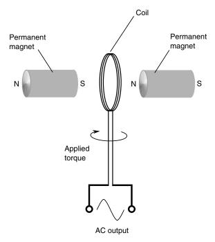
Fig. 14-9. A simple type of ac generator.
