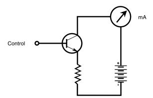
**Fig. 16-7.** Typical biasing of an *npn* transistor.
