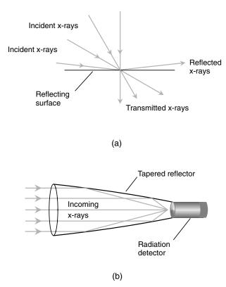
**Fig. 18-7.** (a) x-rays are reflected from a surface only when they strike at a grazing angle. (b) A functional diagram of an x-ray focusing and observing device.
