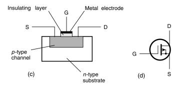
**Fig. 16-14.** Pictorial diagram of an *n*-channel MOSFET (*a*), schematic symbol for an *n*-channel MOSFET (*b*), pictorial diagram of a *p*-channel MOSFET (*c*), and schematic symbol for a *p*-channel MOSFET (*d*).
