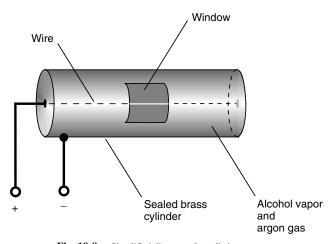
**Fig. 18-8.** Simplified diagram of a radiation counter.
