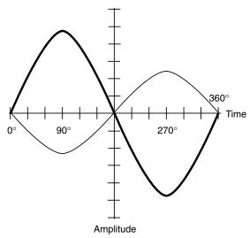
Fig. 13-14. Two sine waves in phase opposition.
