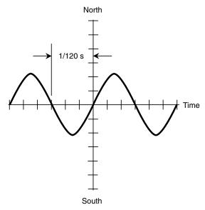
Fig. 14-5. Polarity change in an ac electromagnet.
