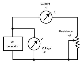
Fig. 12-8. Circuit for working Ohm's law problems.
