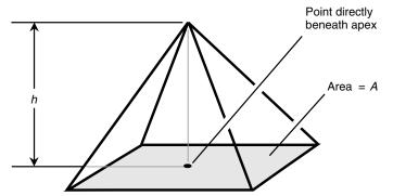
Fig. 4-35 Volume of a pyramid.
