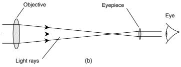
**Fig. 19-10.** The galilean refractor (a) uses a convex objective and a concave eyepiece. The keplerian refractor (b) has a convex objective and a convex eyepiece.
