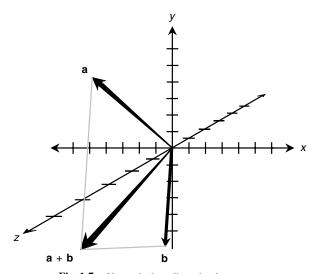
**Fig. 1-7.** Vectors in three-dimensional *xyz* space.
