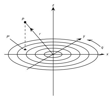
Fig. 3-16. Cylindrical coordinates for defining points in three-space.
