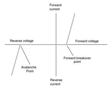
Fig. 16-3. Characteristic curve for a semiconductor diode.
