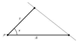
Fig. 4-16 Side-angle-side triangles.
