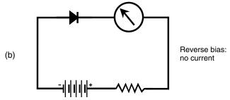
**Fig. 16-2.** (*a*) Forward bias of a diode results in a flow of current. (*b*) Reverse bias normally produces near-zero current.
