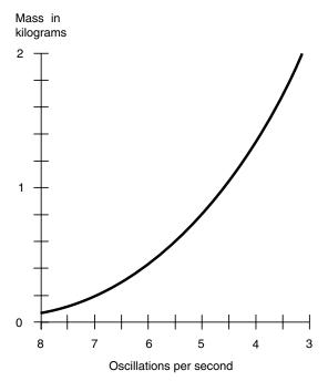
**Fig. 7.2.** Graph of mass versus oscillation frequency for a hypothetical "mass meter" such as the one shown in Fig. 7-1.
