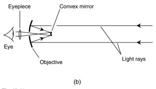
**Fig. 19-11.** The newtonian reflector (a) has an eyepiece set into the side of the tube. In the cassegrain reflector (b), the eyepiece is in the center of the objective mirror.
