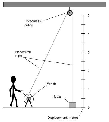
Fig. 8-5. Illustration of power. A winch and pulley can be used to life a heavy object.
