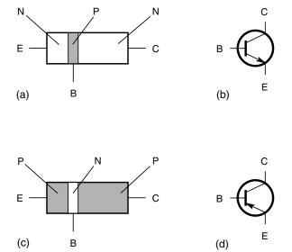
**Fig. 16-6.** Pictorial diagram of *npn* transistor (*a*), schematic symbol for *npn* transistor (*b*), pictorial diagram of *pnp* transistor (*c*), and schematic symbol for *pnp* transistor (*d*).
