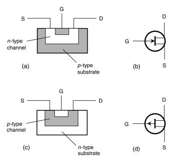
**Fig. 16-10.** Pictorial diagram of an n-channel JFET (a), schematic symbol for an n-channel JFET (b), pictorial diagram of a p-channel JFET (c), and schematic symbol for a p-channel JFET (d).
