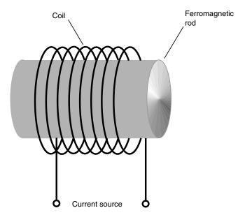
Fig. 14-4. A simple electromagnet.
