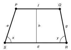
Fig. 4-32 Perimeter and area of a trapezoid.
