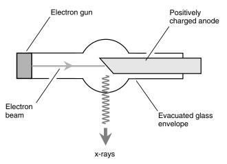
Fig. 18-6. Functional diagram of an x-ray tube.
