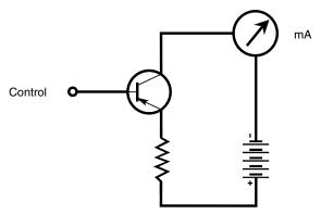
Fig. 16-9. Typical biasing of a pnp transistor.
