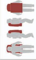
The EMU contains a pack, worn on the back, called the Primary Life Support Subsystem. It holds equipment for oxygen supply, carbon dioxide removal, two-way communication, and water-cooling, as well as an electricity supply and a fan.
