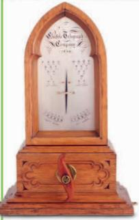
Long-distance communicator This is a single-needle electric telegraph machine, which later developed into double-needle and four-needle instruments.
