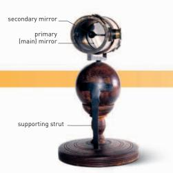
Newton's telescope (front view)
