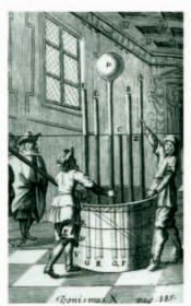
Torricelli's barometer In this engraving, Torricelli demonstrates the existence of atmospheric pressure through the use of mercury-filled tubes.
