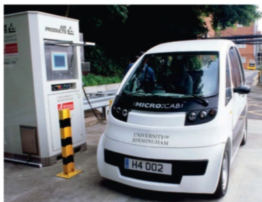
Above: A hydrogen-powered vehicle being refuelled with hydrogen at an experimental filling station. Inside the car, a fuel cell produces electrical power from the reaction of hydrogen with oxygen.
