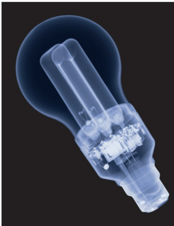
Above: X-ray image of a compact fluorescent lamp. The glass tubes inside the bulb are filled with mercury vapour, which produces ultraviolet radiation when electric current flows through it; the ultraviolet excites phosphors on the inner surface of the tubes, which emit visible light.
