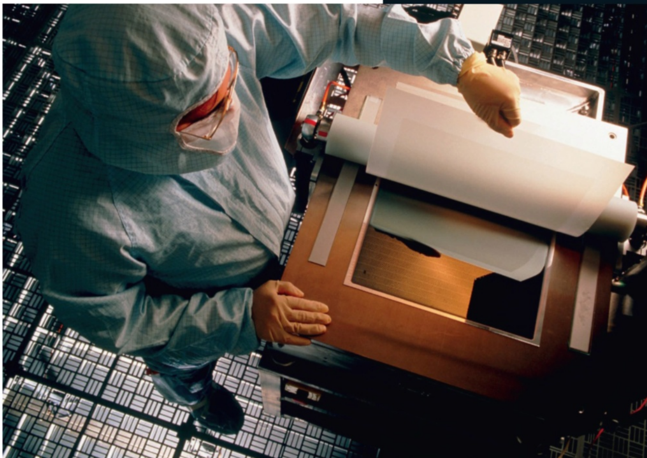
Below: Technician preparing a plate for use in a digital X-ray imaging device. The plate is made of glass and is coated with selenium, which produces electrons when X-ray photons strike it
