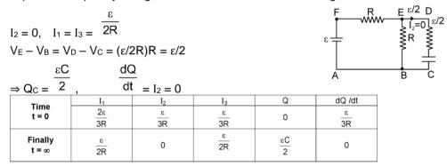
**Example 6.** At t = 0 switch  $S_1$  is closed and remains closed for a long time and  $S_2$  remains open. Now  $S_1$  is opened and  $S_2$  is closed. Find out
