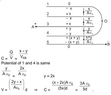
Five similar condenser plates, each of area A, are placed at equal distance d apart and are Problem 10. connected to a source of e.m.f. V as shown in the following diagram. The charge on the plates 1 and 4 will be-
