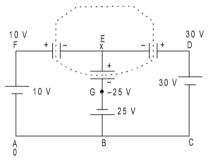
Let potential at A is 0, so at D it is 30 V, at F it is 10 V and at point G potential is -25V. Now apply kirchhoff's I<sub>st</sub> law at point E. (total charge of all the plates connected to 'E' must be same as before i.e. 0)
