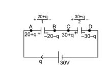
Charge on capacitor of capacitance  $1\mu F = 20 + q = \frac{3}{80} \mu C$
