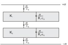
(vi) Comparison of E (electric field), σ (surface charges density), Q (charge), C (capacitance) and before and after inserting a dielectric slab between the plates of a parallel plate capacitor.
