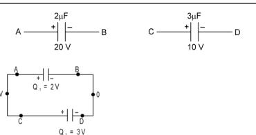
Let potential of B and D is zero and common potential on capacitors is V, then at A and C it will be V.
