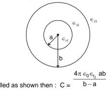
If dielectric mediums are filled as shown then : C = **Cylindrical capacitor**
