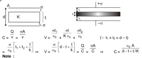
(i) Capacitance does not depend upon the position of dielectric (it can be shifted up or down still capacitance does not change).
