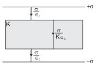
The total electric field produced by bound induced charge on the dielectric outside the slab is zero because they cancel each other.
