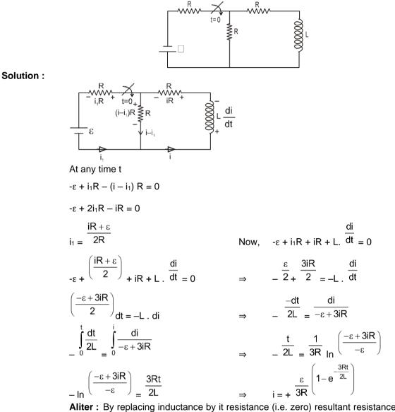
Aliter : By replacing inductance by it resistance (i.e. zero) resultant resistance of circuit is 3R/2so Imax through battery is Imax =  $\frac{2\epsilon}{3R}$ ,
