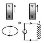
On moving the south pole of a magnet away from the coil the current induced in the coil will appear flowing in the anticlockwise direction as seen from the side of magnet and the face of the coil towards the magnet will behave like a north pole.
