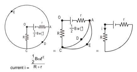
**Example 18.** Solve the above question if the length of rod is 2L and resistance 2r and it is rotating about its centre. Both ends of the rod now touch the conducting ring
