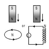
On bringing a south pole towards a coil the current induced in the coil will appear flowing in clockwise direction as observed from the side of magnet and the face of the coil towards the magnet will behave as a south pole.
