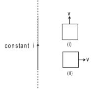
**Solution :** In loop (i) no emf will be induced because there is no flux change. In loop (ii) emf will be induced because the coil is moving in a region of decreasing magneticfield inward in direction. Therefore to oppose the flux decrease in inward direction, current will be induced such that its magnetic field will be inwards. For this direction of current should be clockwise.
