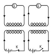
When current is passed through a coil, the current flowing through the coil changes. As a result the magnetic flux linked with the coil changes. Due to this a current is induced in the coil. If the current induced in the coil flows in the opposite direction of the applied current. If the current flowing in the coil is decreased, then the current induced in the coil flows in the direction of the applied current so as to oppose the decrement of the applied current.
