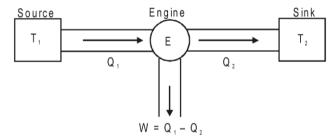
Engine derives an amount 'Q<sub>1</sub>' of heat from the source.
