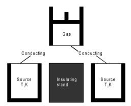
**Source :** It is a reservoir of heat energy with a condicting top maintained at a constant temperature T<sub>1</sub>K. Source is so big that extraction of any amount of heat from it does not change its temperature.
