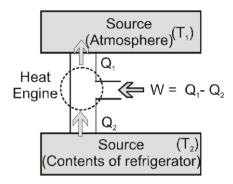
The working substance takes heat  $Q_2$  from a sink (contents of refrigerator) at lower temperature, has a net wmount of worj done W in it by an external agent (uaually compressor of refrigerator) and gives out a larger amount of heat  $Q_1$  to a hot body at temperature  $T_1$  (usally atmosphere) Thus, it transfers heat form a cold to a hot body at the expense of mechanical energy supplied to it by an external agent. The cold is thus cooled more and more.
