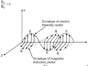
In figure, electric field vector <sup>(E)</sup> and magnetic field vector <sup>(B)</sup> are vibrating along Y and Z directions and propagation of electromagnetic wave is shown in X-direction. Hence, electric and magnetic fields are in phase and perpendicular to each other.
