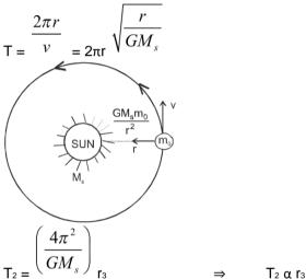
For all the planet of a sun ,  $T_2 \propto r_3$
