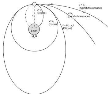
Suppose a stallite is at a distance r from the centre of the earth. If we give different velocities (v) to the satellite, its path will be different
