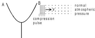
After producing the compression pulse, the prong B reverses its motion and moves inward. This drags away some air from the region in front of it, causing the pressure to dip slightly below the normal pressure. This region of decreased pressure is called a rarefaction pulse. Following immediately behind the compression pulse, the rarefaction pulse also travels away from the prong with the speed of sound.
