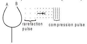
If the prongs vibrate in SHM, the pressure variations in the layer close to the prong also varies simple harmonically and hence increase in pressure above normal value can be written as
