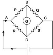
In the wheat stone bridge :  $\frac{P}{If} = \frac{R}{S} + \frac{P}{S} = V_D \quad But \text{ if } \quad \frac{P}{Q} > \frac{R}{S}$ then potential drop across P will be more than that across R. So potential at B will be less than that at D. So current in the Galvanometer
