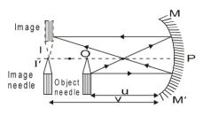
First of all we make a rough estimation of f. For estimating f roughly, make a sharp image of a far away object (like sun) on a filter paper. The image distance of the far object will be an approx estimation of focal length.
