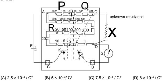
17.\* In the meter bridge circuit, the point D is the balance point.
