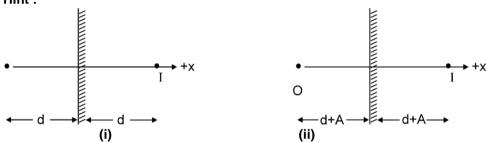
From figure (i) and (ii) it is clear that if the mirror moves distance 'A' then the image moves a distance '2A'.
