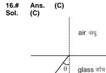
Initially most of part will be transmitted. When  $\theta > i_C$ , all the light rays will be total internal reflected. So transmitted intensity = 0 So correct answer is (C)
