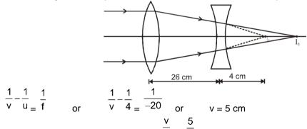
magnification for concave lens m = u = 4 = 1.25As size of the image at  $I_1$  is 2 cm. Therefore, size image at  $I_2$  will be 2 × 1.25 = 2.5 cm.
