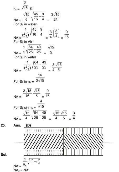
Therefore the numerical aperture of combined structure is equal to the lesser of the two numerical aperture, which is  $NA_2$
