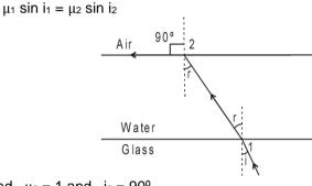
Here  $\mu_1 = \mu_g$ ; and  $\mu_2 = 1$  and  $i_2 = 90^{\circ}$  $i_1 = i$  $\mu_g \sin i = (1) (\sin 90^{\circ})$ or  $\mu_g = \frac{1}{\sin i}$
