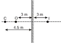
From diagram distance of camera from image = 4.5 + 3 = 7.5 m.
