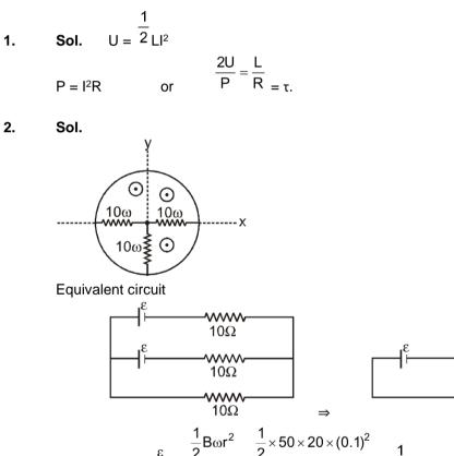
So current  $I = \frac{\varepsilon}{R} = \frac{\overline{2}^{Bor}}{15} = \frac{\overline{2}^{\times 50 \times 20 \times (0.1)}}{15} = \frac{1}{3} \text{Amp.}$
