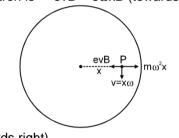
Centrifugal force =  $m\omega^2 x$ . (towards right) For net force on the electron at P to be zero  $e\omega x B = m\omega^2 x$ i.e..
