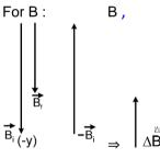
The change in the magnetic field which causes induced current  $(\Delta \tilde{B})$  is along (+)z direction.
