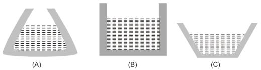
(7) In a liquid at same level, the pressure will be same at all points, if not, due to pressure difference the liquid cannot be at rest. This is why the height of liquid is the same in vessels of different shapes containing different amounts of the same liquid at rest when they are in communication with each other.
