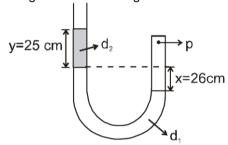
**Solution :** Pressure in a liquid at same level is same i.e. at A - A -,  $p_a + d_2yg + xd_1g = p$
