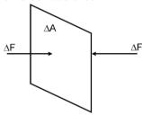
The pressure is a scalar quantity. This is because hydrostatic pressure is transmitted equally in all directions when force is applied, which shows that a definite direction is not associated with pressure.
