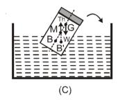
However, if meta-centre goes CG, the couple due to forces at G and B' tends to topple the floating body. That is why a wooden log cannot be made to float vertical in water or a boat is likely to capsize if the sitting passengers stand on it. In these situations CG becomes higher than MG and so the body will topple if slightly tilted.
