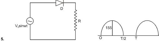
$$V_{ms} = \frac{\left(\frac{V_0}{2}\right) = \frac{155}{2} = 77.5 \text{ volt}}{V_{0} = \frac{310}{2}} = 155 \text{ volt.}$$
