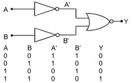
Output of this is same as that of AND gate. Alternatively The Boolean expression for the given logic gate is  $\underline{-----}$
