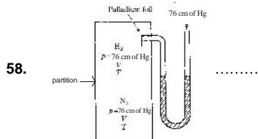
**Sol.** The lower compartment contains N<sub>2</sub> (which cannot pass the Pd foil) under 76 cm of Hg pressure. After removing partition, the hydrogen behave exactly as if the N<sub>2</sub> were not present since the volume available to the H<sub>2</sub> has doubled, the pressure in the container has fallen to one half its original value.
