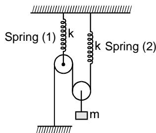
Initially the block is at rest under action of force  $2T$  upward and  $mg$  downwards. When the block is pulled downwards by  $x$ , the spring (1) extends by  $x_1$  and spring (2) extends by  $x_2$ .
