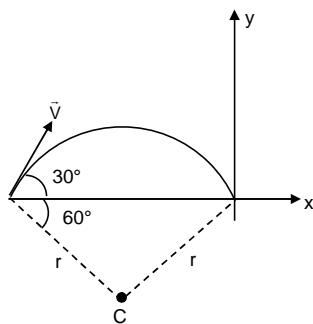
As  $\vec{V} \perp \vec{B}$  particle will follow circular path of radius
