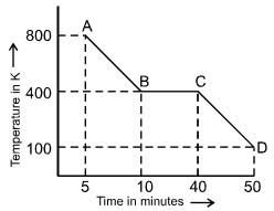
AB represent cooling of liquid, BC represent conversion of liquid to solid, CD represent cooling of solid. The molar entropy of fusion in J mole<sup>-1</sup>  $K^{-1}$  is (Give your answer after dividing by 10):
