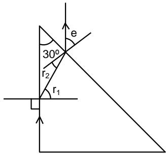
$$\frac{\sin 90^\circ}{\sin r_1} = \mu = \frac{1}{\sin 42^\circ} \Rightarrow r_1 = 42^\circ$$
