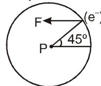
$$\therefore \text{acceleration of electron } a_e = \frac{\rho ae}{3\epsilon_0 m}$$
