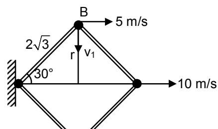
$$\text{speed of D} = \sqrt{5^2 + v_1^2 + (\omega r)^2}$$
