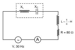
34. In the LCR circuit shown if only L is removed, the current leads the supply voltage by 30°. If only C is removed, the current lags the voltage by 60°. The resonant frequency is  $\frac{50x}{\sqrt{3}\pi}$  Hz, then write the value of 'x'.
