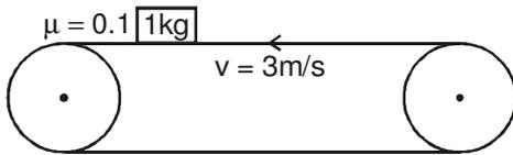
Maximum heat liberated then all kinetic energy is loss in heat due to friction
