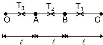
$$T_1 = m\omega^2 R = m\omega^2 (3l) \dots(1)$$
