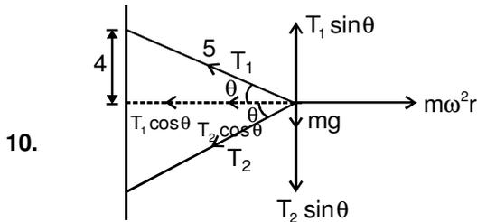
$\Rightarrow T_1 \cos \theta + T_2 \cos \theta = m \omega^2 r \quad \dots(1)$
