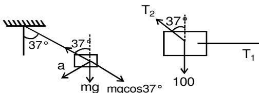
$$T_2 \times \frac{4}{5} = 100 \quad T_1 = 80 \text{ N}$$
