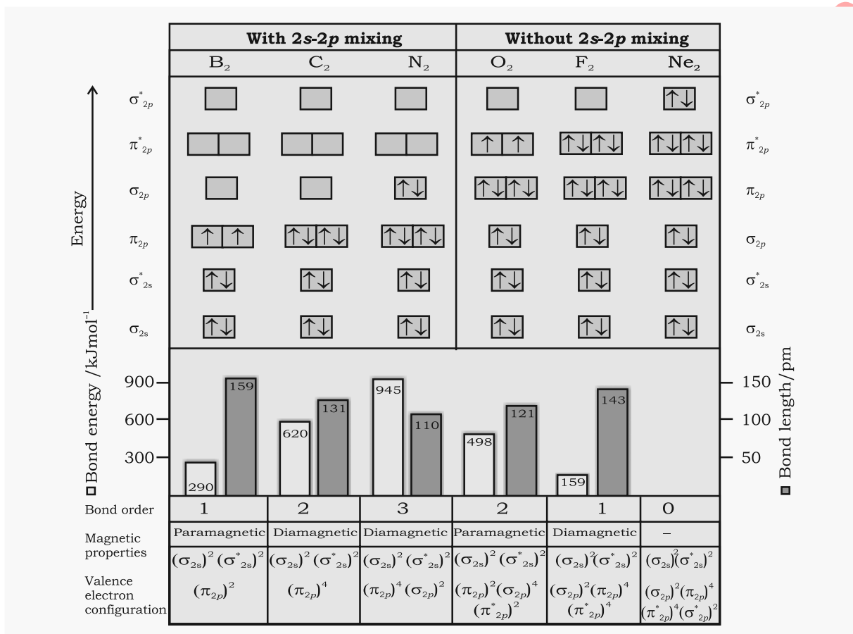
Fig. 4.21 MO occupancy and molecular properties for B 2 through Ne 2 .
