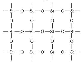
Fig. 11.6 Three dimensional structure of SiO<sub>2</sub>
