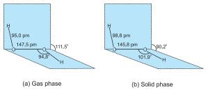
**Fig. 9.3** (a)  $H_2O_2$  structure in gas phase, dihedral angle is  $111.5^{\circ}$ . (b)  $H_2O_2$  structure in solid phase at 110K, dihedral angle is  $90.2^{\circ}$ .
