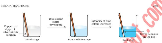
Fig. 8.2 Redox reaction between copper and aqueous solution of silver nitrate occurring in a beaker.
