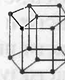
Hexagonal Primitive a = b \neq c \alpha = \beta = 90^\circ, \gamma = 120^\circ
