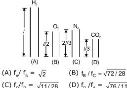
17. A gas is filled in an organ pipe and it is sounded with an organ pipe in fundamental mode. Choose the correct statement(s) : (T =constant)
