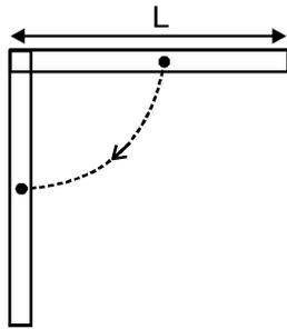
$$Mg \frac{L}{2} = \frac{1}{2} I\omega^2, \quad \omega = \sqrt{\frac{3Mg\ell}{ML^2}} = \sqrt{\frac{3g}{L}}$$
