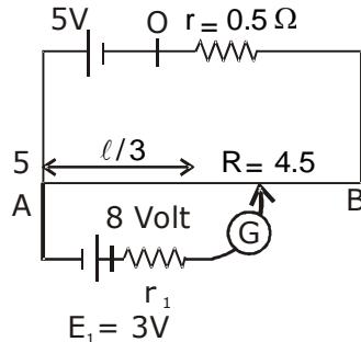
As Battery is connected in reverse order  $E_1$  will not be balanced on entire length of wire AB.
