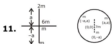
$$Y_{\text{com}} = \frac{2m(+a) + 6m(0) + m(0) + m(-a)}{2m + 6m + m + m}$$
