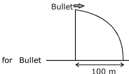
$$X_{\text{Bullet}} = V_{\text{Bullet}} \times \sqrt{\frac{2H}{g}}$$
