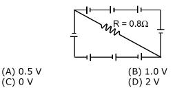
28. In the circuit shown, what is the potential difference  $V_{PO}$  ?
