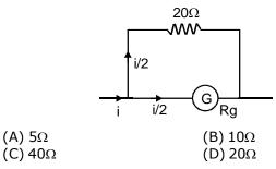
**80.** A galvanometer has a resistance of  $20\Omega$  and reads full-scale when 0.2 V is applied across it. To convert it into a 10 A ammeter, the galvanometer coil should have a
