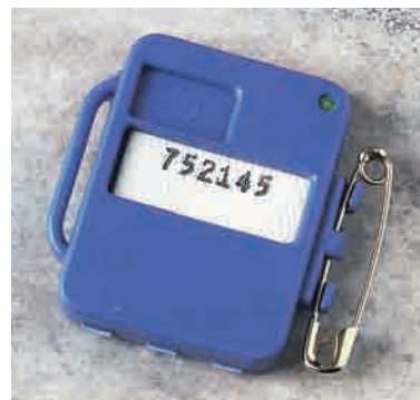
Figure 13.15 This badge indicates the amount of radiation received by its wearer.
