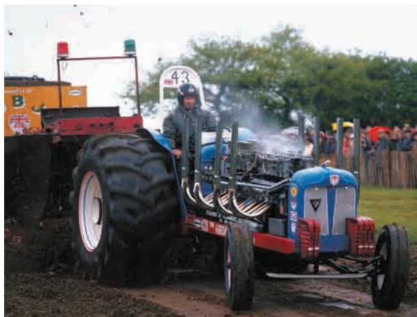
Figure 1.5 In a tractor pull, vehicles develop up to 9000 horsepower to accelerate a sled, until they can no longer overcome the constantly increasing frictional forces. Dragsters, on the other hand, accelerate right up to the finish line.
