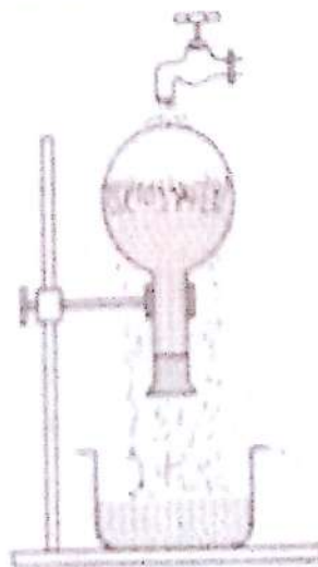
Fig. 11.15 Water boils below 100^{\circ}\text{C} under reduced pressure.
