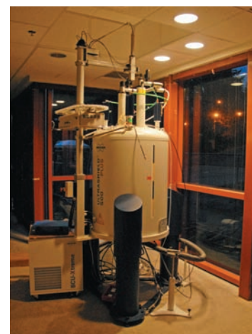
The superconducting magnet of an FTNMR spectrometer.
