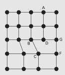
**Dislocation in a two-dimensional crystal**. The extra plane of atoms AB causes strain at bond CD. On breaking, the bond flips across to form CB. This incremental movement shifts the dislocation across so that the overall effect is to slide the two planes BDG and CF over each other.
