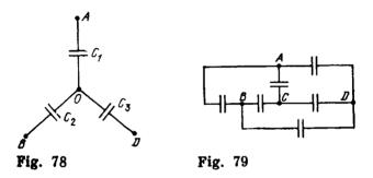
3.13. Where must a current source be connected to the circuit shown in Fig. 79 in order to charge all the six capacitors having equal capacitances?
