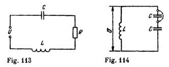
included in the circuit shown in Fig. 113 is charged to  $q_1 = 10^{-9}$  C. The inductance of the coil is  $L = 10^{-5}$  H, and the resistance of the resistor is R = 100  $\Omega$ .
