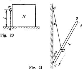
For what mass ratio M/m will the rod form an angle  $\alpha = \pi/6$  with the horizontal at the moment of the separation from the body? What will be the velocity u of the body at this moment? Friction should be neglected.
