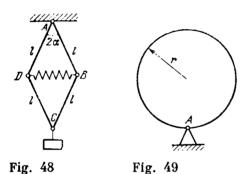
1.97. A thin hoop is hinged at point A so that at the initial moment its centre of mass is almost above point A (Fig. 49). Then the hoop is smoothly released, and in a time  $\tau = 0.5$  s, its centre of mass occupies the lowest position.
