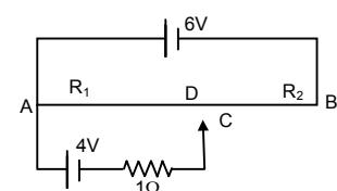
c) When the points C and D are connected by a wire current flowing through it is 0 since the points are equipotential.
