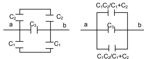
17. In the figure the three capacitors are arranged in parallel.
