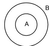
$$\left(\frac{E}{t}\right)_A = \sigma A_A [(373)^4 - (293)^4] \Rightarrow (mS)_A \left(\frac{d\theta}{dt}\right)_A = \sigma A_A [(373)^4 - (293)^4]$$
