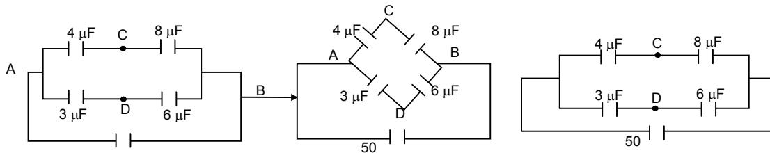
$$(a) \text{Capacitor} = \frac{4 \times 8}{4+8} = \frac{8}{3} \mu\text{F}$$
