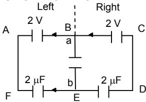
From the figure it is cleared that the left and right branch are symmetry and reversed, so the current go towards BE from BAFEB same as the current from EDCBE.
