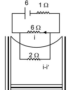
$$(a) \text{Heat} = i^2 RT = \frac{9}{5} \times \frac{9}{5} \times 2 \times 15 \times 60 = 5832$$
