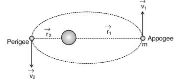
In case of elliptical orbit, the speed of satellite varies constantly as shown in figure. Thus according to the law of conservation of angular momentum, the satellite must move faster at a point of closest approach (Perigee) than at a farthest point (Appogee).
