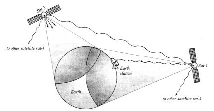
First the information is sent to the nearest satellite in the range of earth station by means of electromanetic waves then that satellite broadcasts the signal to the region of earth exposed to this satellite and also send the same signal to other satellite for broadcasting in other parts of the globe.
