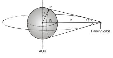
During revolution satellite leaves two spherical patches 1 and 2 on earth surface at north and south poles where no signals can be transmitted due to curvature. The areas of these patches can be obtained by solid angles.
