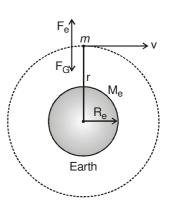
As gravitational force on satellite due to earth is the only force it experiences during motion, it has gravitational interaction energy in the field of earth, which is given as
