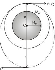
As the particle velocity is greater than the velocity required for circular orbit, hence the particle path deviates from circular path to elliptical path. At position of minimum and maximum distance velocity vectors are perpendicular to instantaneous radius vector. In this elliptical path the minimum distance of particle from earth's centre is a and maximum speed in the path is v<sub>p</sub> and let the maximum distance and minimum speed in the path is r and  $v_1$  respectively.
