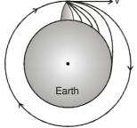
Let's find the speed of a satellite of mass *m* in a circular orbit around the earth. Consider a satellite revolving around the earth in a circular orbit of radius r as shown in figure. If its orbit is stable during its motion, the net gravitational force on it must be balanced by the centrifugal force on it relative to the rotating frame as
