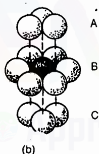
Figure 2.5 Arrangement of 12 neighbours in hexagonal close-packed and cubic close-packed structures. (Note that the top and bottom layers are the same, the cubic close-packed structure is 60° relative to the hexagonal close-packed.) (a) Hexagonal close-packed. (b) Cubic close-packed.
