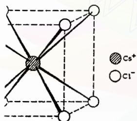
3.6 Caesium chloride structure. (Reproduced by permission of Wells, A.F., Inorganic Chemistry , Oxford University Press, 1984.)
