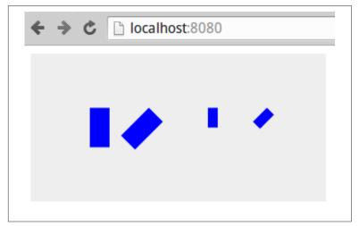
Figure 4-15. Some SVG transforms: rotate(45), scale(0.5), scale(0.5) +rotate(45)
