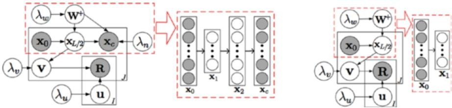
**Figure 7-2.** Scheme of a possible collaborative deep learning model. On the left is the graphical model. The dashed rectangle represents an auto-encoder. On the right is the graphical model of the degenerated model. The dashed rectangle represents the encoder component of SDAE (source: [www.wanghao.in/paper/KDD15\\_CD\\_L.pdf](http://www.wanghao.in/paper/KDD15_CD_L.pdf)).
