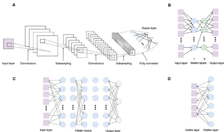
**Figure 3-3.** Four of the most popular classes of deep learning architectures in data analysis. A. A CNN has several levels of convolutional and subsampling layers optionally followed by fully connected layers with deep architecture. B. The stacked auto-encoder consisting of multiple sparse auto-encoders. C. A DBN is trained layer-wise by freezing previous layer weights and feeding the output to the next layer. D. The RBM architecture includes one visible layer and one layer of hidden units.
