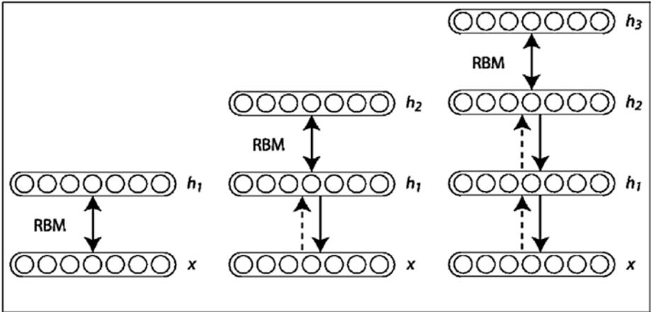
**Figure 3-5.** Illustration of deep belief networks. The bottom layers (all layers except the top one) do not have the bidirectional connections, but only connections from the top down.
