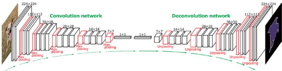
**Figure 4-2.** Example of a fully convolutional neural network for image segmentation (source: [https://handong1587.github.io/deep\\_learning/2015/10/09/segmentation.html](https://handong1587.github.io/deep_learning/2015/10/09/segmentation.html))
