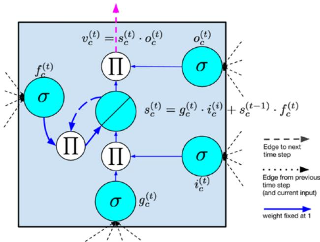
**Figure 3-9.** An LSTM cell with forgetting memory gate (source: <https://arxiv.org/pdf/1506.00019.pdf>)
