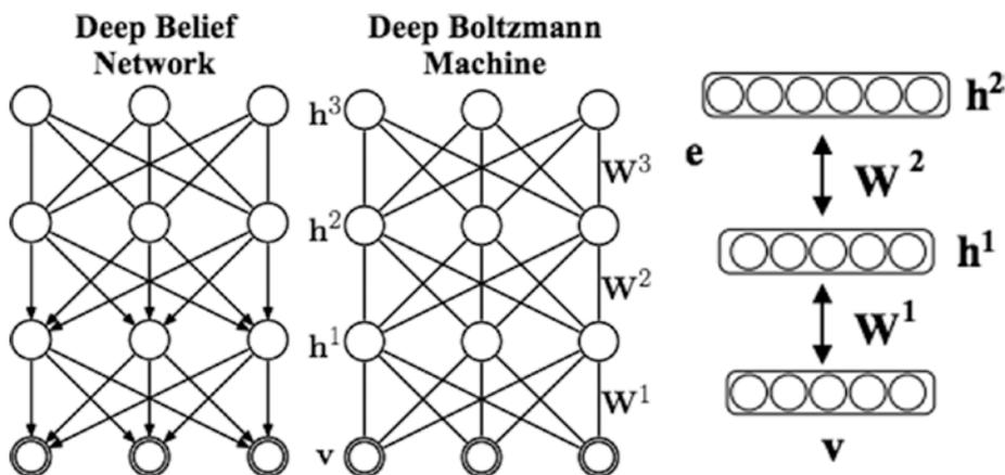
**Figure 3-6.** Illustration of deep Boltzmann machine (DBM). The deep Boltzmann machine is more like stacking RBMs together. Connections between every two layers are bidirectional (source: [www.cs.toronto.edu/~rsalakhu/DBM.jpg](http://www.cs.toronto.edu/~rsalakhu/DBM.jpg)).
