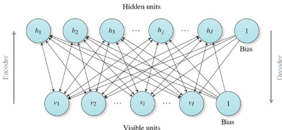
**Figure 3-4.** Illustration of restricted Boltzmann machine. With the restriction that there are no connections between hidden units ( $h_j = 1 \dots J$  nodes) and no connections between visible units ( $v_i = 1 \dots I$  nodes), the Boltzmann machine turns into a restricted Boltzmann machine. The model now is a bipartite graph.
