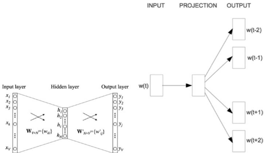
**Figure 5-2.** Left: Representation of a Siamese network behind the Word2vec model. The hidden nodes  $h_1, \dots, h_N$  contain the vectorized representation of the word. Right: The schematic representation of word2vec using a skip-gram (word  $W(t)$  is used to predict context words  $W(t-2) \dots W(t+2)$ ). Here a context window of  $K = 5$  is considered (source: <https://stackoverflow.com/questions/30835737/word2vec-data-setup>).
