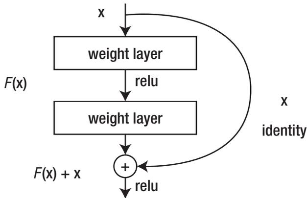
**Figure 4-5.** Architecture of a residual network (source: <https://arxiv.org/abs/1512.03385>)
