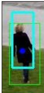
In this screenshot, the blue rectangle is the CAMShift detection and the green rectangle is the Kalman filter prediction with its center at the blue circle.
