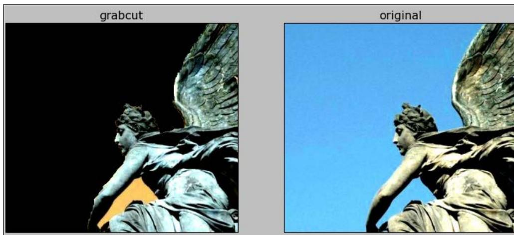
This is quite a satisfactory result. You'll notice that an area of background is left under the angel's arm. It is possible to apply touch strokes to apply more iterations; the technique is quite well illustrated in the `grabcut.py` file in `samples/python2` of your OpenCV installation.
