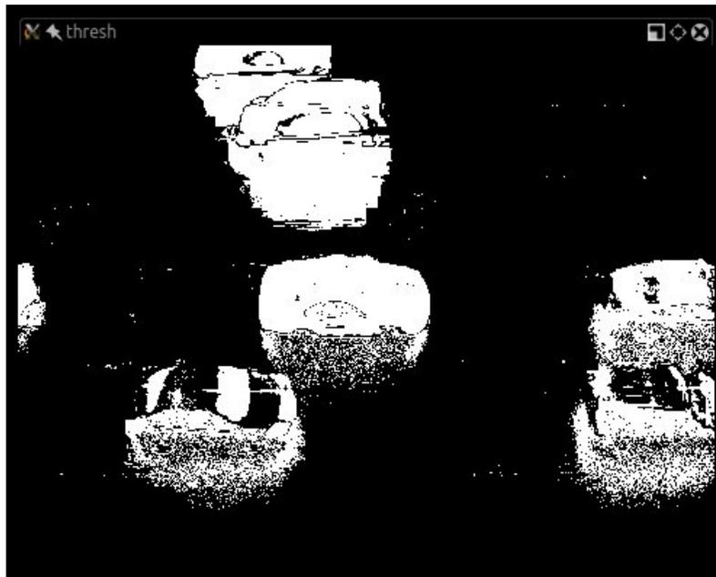
Here's an example of shadow detection (with shadows thresholded):
